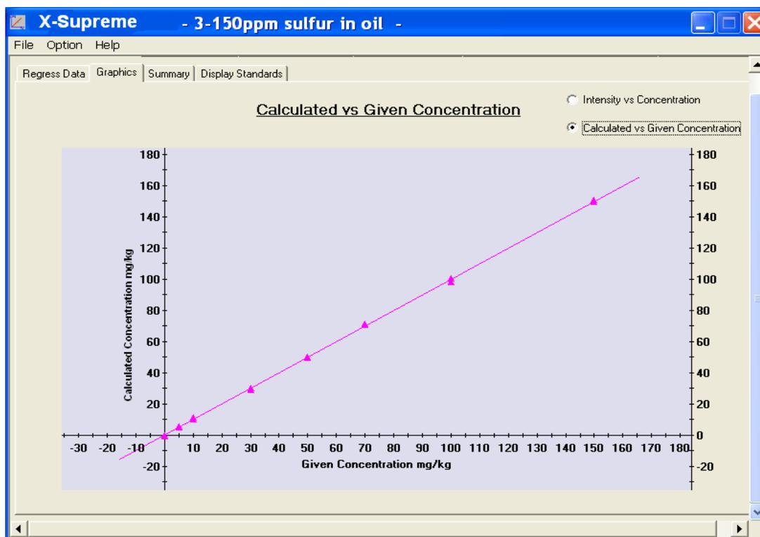
Figure 3: Ultra low sulfur calibration
